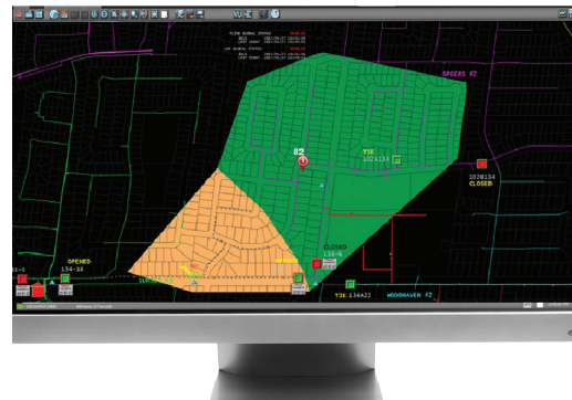
FLISR (Fault Locations, Isolation and Service Restoration) shown on a monitoring computer
